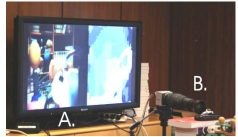
Figure 2. The CAFADIS camera. (A) Result of 3D reconstruction shown as color+depth image on a Philips 3D display. (B) The CAFADIS camera recording the scene.
