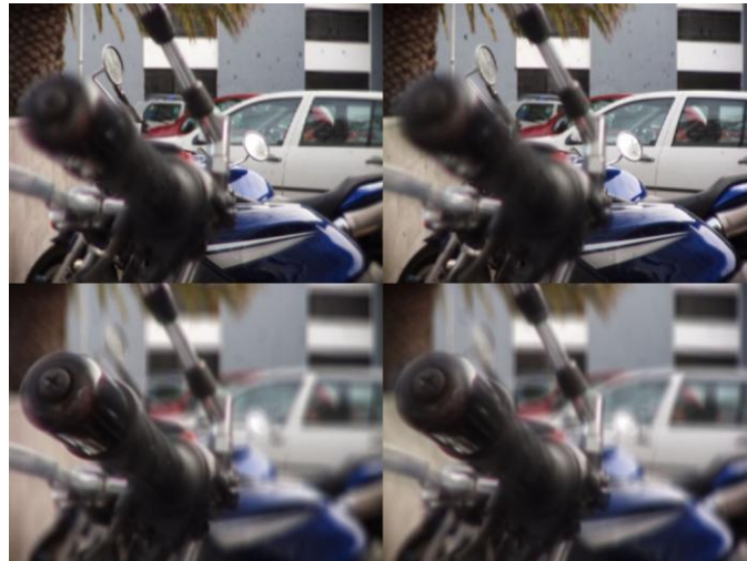
Figure 6. A pair of stereo images digitally focused at two different depths with our technology.
